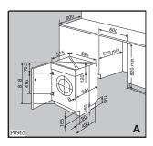
When installing the appliance into the kitchen furniture ensure, if possible, the hoses are placed in either of the two recesses on the back of the appliance. This will help to prevent the hoses from becoming kinked or trapped. Picture AB.
